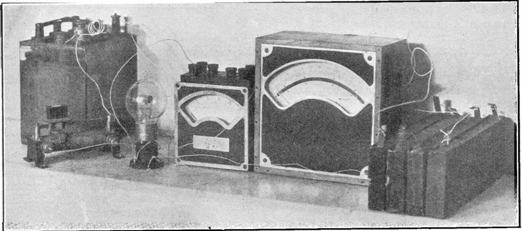
Photograph of the apparatus connected to obtain voltage saturation curves. The connections are given in Fig. 3.
